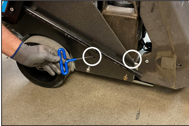
Loosening middle weight locking screws.
