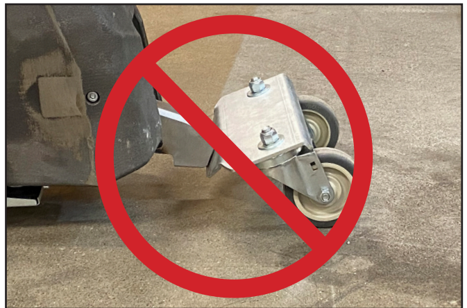
Poor maneuverability--bracket NOT parallel to floor.
