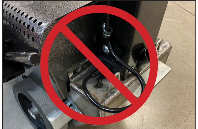
Power cord should NOT have excess slack.
