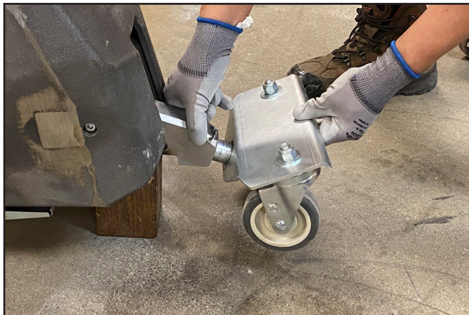
Installing transport wheels.
