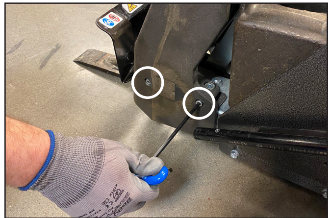
Loosening front weight locking screws. (Right side not shown.)
