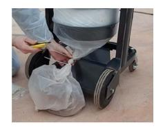
> Pull down a length of new bag from the chamber, until it reaches the bottom support plate
