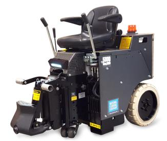
Ensure the seat is securely fastened to the machine. The seat has a safety switch. The operator must be properly seated for the machine to run.
