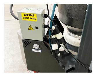
6. Plug the main power cord into the power supply.
