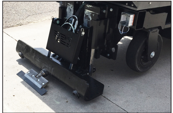
Decreased blade tilt angle and raised blade. Front caster wheels off ground.
