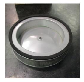
406313 - COMPRESSOR AIR FILTER WITH CARTRIDGE
